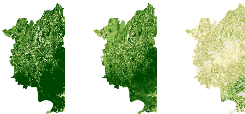
Figure - 2. Representative NDVI maps of Almaty City for June, September, November 2020. Sentinel-2 L2A NDVI composites with cloud coverage <30%. Note: Compiled by the authors based on [3; 21]
